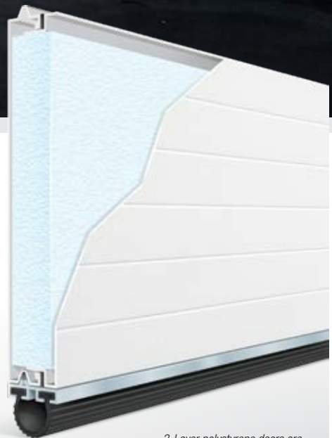
3-Layer polystyrene doors are 2" or 1-3/8" sandwich construction
